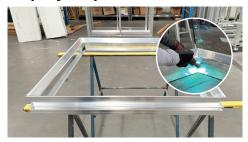
1 Pre-Step: Soldering four pieces of the main frame to create a square frame.
