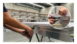
4 Tight tension on the right side & the left side using a clamp, then secure it with a screw.
