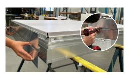
7 Fitting the full or half cover on each edge and then secure it with a screw (Four sides).
